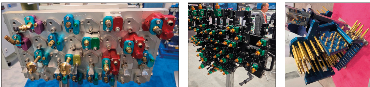
Figure 17 : exemples de poteyeurs (AED Automation, Bohmer, Gerlieva)
