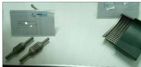
Fig.28 – Structures lattices issues de fabrication additive (RWTH Aachen)
